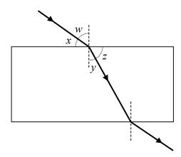
A student uses the equation  $_1\mu_2 = \frac{\sin i}{\sin r}$  to calculate the refractive index.
